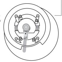
Turn the dripper cone upside down and remove the four screws in the base using a Phillips-head screw driver. Then remove the center of the base, exposing the lever mechanism.
